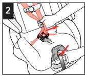
Loosen harness by pushing down on the harness release lever while pulling out on harness.
